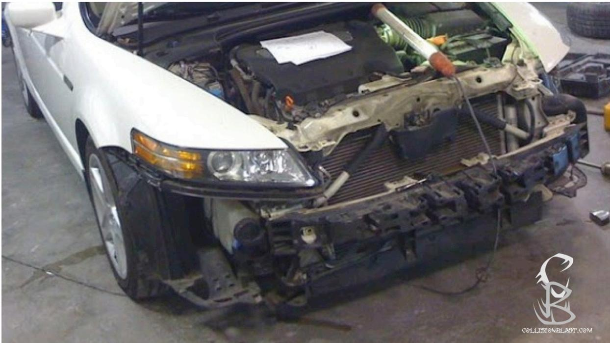
An example of removing the bumper cover to inspect hidden damage.
