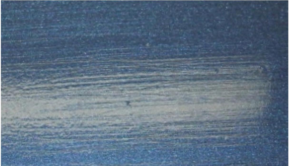
Photo of sand scratch swelling. A sign of previous body work.
