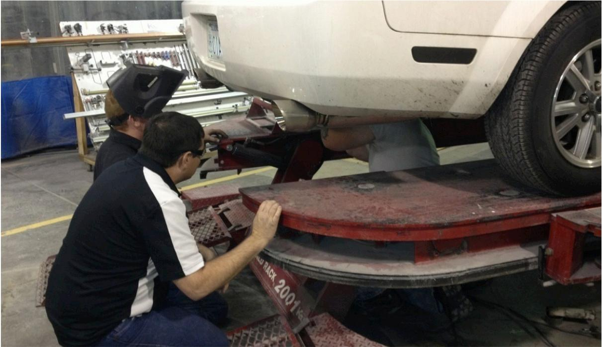
Inspecting underneath the vehicle for structural damage.
