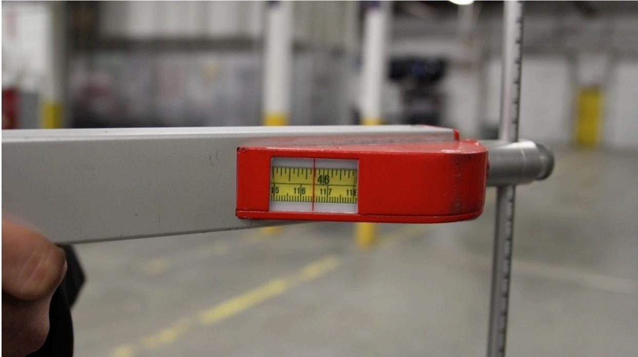
This is an example of a tram gauge used for point to point measurements.
