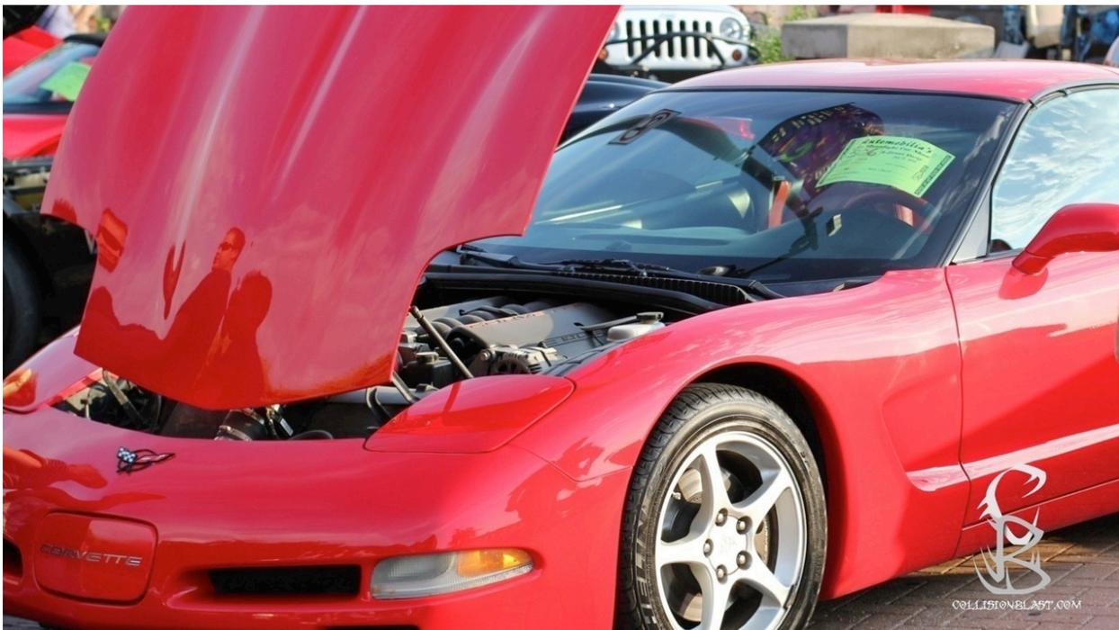
Corvettes have been made with different composite through the years. Starting with fiberglass, then SMC, and now carbon fiber.
